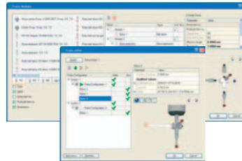
The measuring results are displayed in a 3D view and can be added including settings, like tolerances, by using drag-and-drop to a measuring report or an export.
