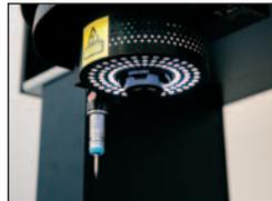
Illumination is essential for accurate measurements. The DeMeet is equipped with LED based illumination (backlight, coaxial light and segmented ringlight).
