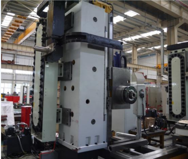
Spindle dia \phi 130 with ATC
