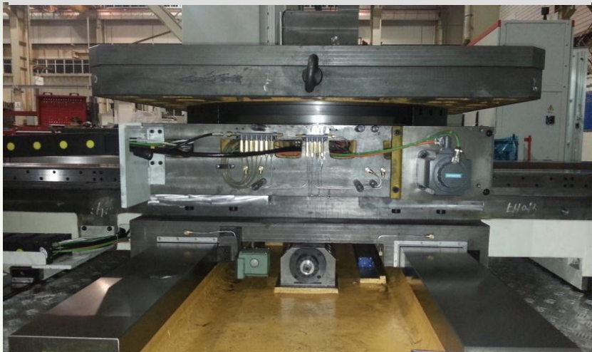
Hydraulic clamping of B axis supplied by independent hydraulic station
