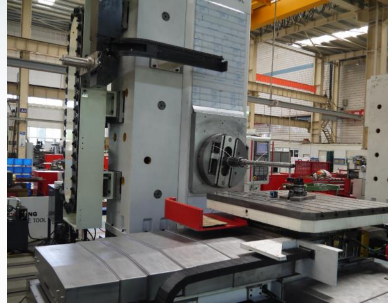
Equipped with facing head and ATC
